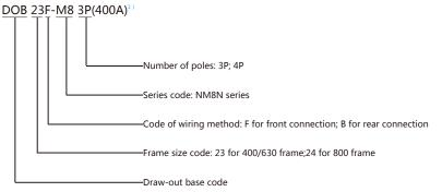
Note<sup>1</sup>): DOB23 is suitable for 400/630 housings. There are two specifications of 400 and 630.
