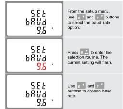
Press E 🕹 to confirm the setting and press 💯 🚅 to return to
