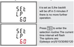
Press M A and P T to select the time interval. Then press to confirm the set-up.
