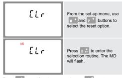
Press E 🕹 to confirm the reset and press 🗤 🚅 to return to the main set up menu.
