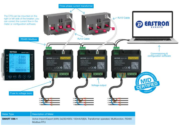
SMART X96-1E Active Import/Export (kWh) 3x230/400V, 100mA/5(6)A, Transformer operated, Multifunction, RS485 Modbus RTU, No THD, No Voltage Output and 1P2W and 3P4W only
