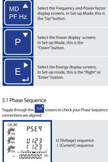
Select the Frequency and Power factor display screens. In Set-up Mode, this is
