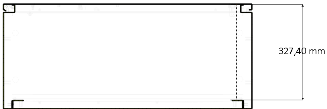
Fig. 5.2. A cross-section picture of the C-series cable distribution cabinet and corresponding installation depth.
