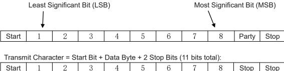
Eastron Digital meters additionally support No parity, One stop bit.
